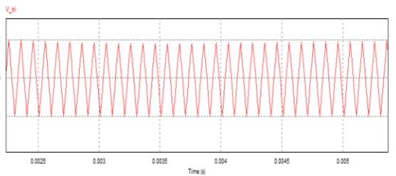
Fig.6.2(b) Triangular waveform
