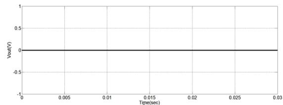
Fig.6.3 (a) output voltage waveform of single phase SPWM inverter with over current protection
