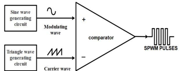
Fig.1 (a) Sinusoidal Pulse Waveform Generation
