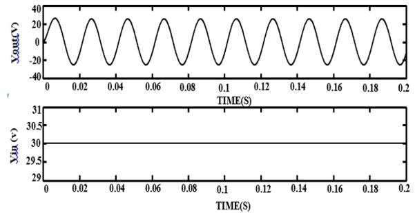
Fig.6.1(a) Input and Output voltage of single phase spwm inverter in open loop system
