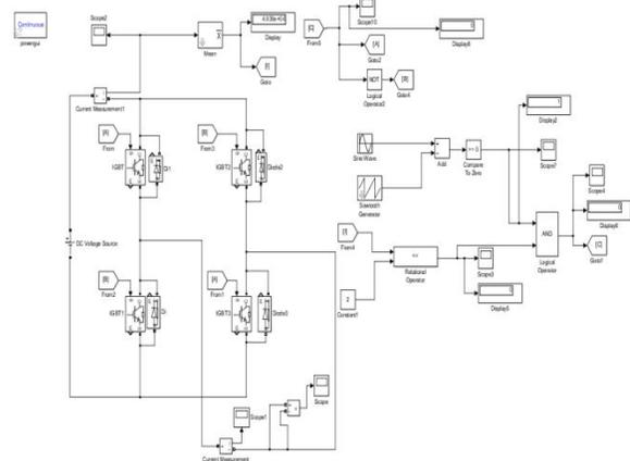
Fig.5(c) single phase SPWM inverter with over current protection
