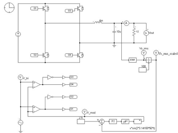
Fig.5 (b) Closed Loop Simulation Diagram
