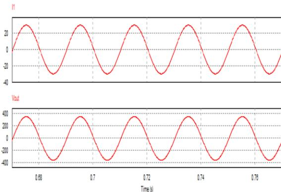
Fig.6.2 (f) output voltage and current waveform of single phase SPWM inverter with filter
