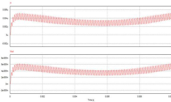
Fig.6.2 (g) Output voltage and current waveform of single phase SPWM inverter in short circuit condition.
