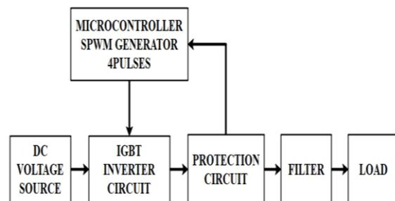
Fig.4 (a) Block diagram of single phase SPWM inverter with protections
