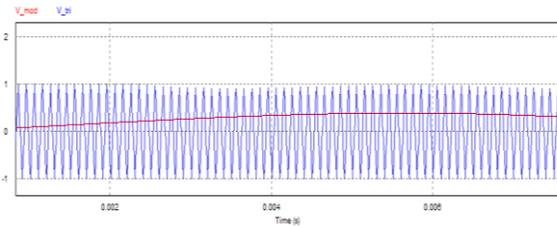
Figure 6.2 (h) sine and triangular wave comparison during short circuit condition
