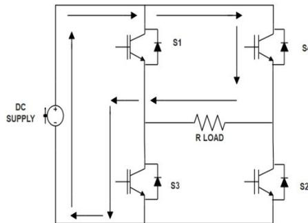
Fig.3 (b) current flow path in Mode 2
