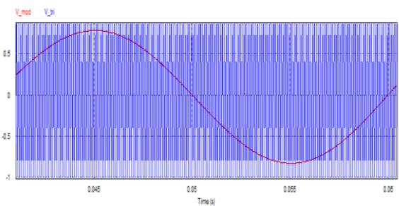
Fig.6.2(c) Sine and Triangular Wave Comparison
