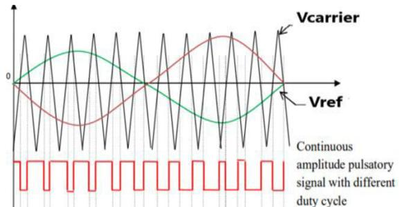
Fig.1 (b) Pulse Waveform
