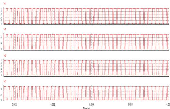
Fig.6 (i) switching pulse waveform during short circuit condition
