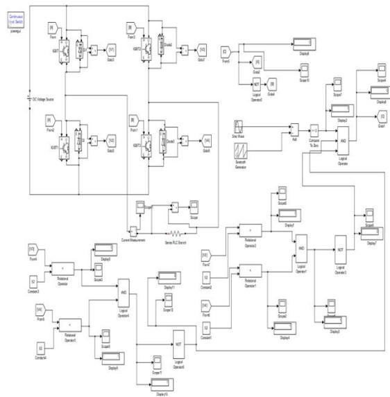
Fig.5(d) single phase SPWM inverter with shoot through fault
